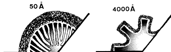
Fig. 6. Schematic representation of the different distribution of the cellulose derivative on the surface of a particle of silica gel depending on the pore size of the matrix.
